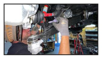
13. Using OE hardware. Re install lower control arms to the 17. Tighten sway bar frame mount. **Torque to 70 ft lbs.** bottom of the steering knuckle. Torque to 140 ft lbs. Repeat on passenger side.
