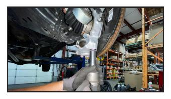
14. Tighten the upper control arm bolts. Torque bolts to 130 ft lbs. Repeat on the passenger side.
