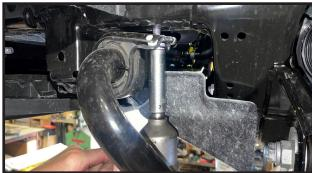
Remove the lower sway bar endlink hardware on the driver and passenger lower control arms.
