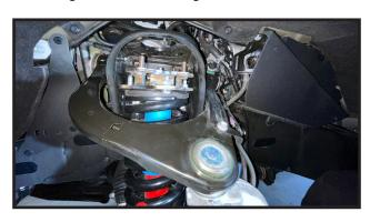
10. Loosen the upper Control arm bolt, on the driver and passenger side to allow it to pivot downwards.
