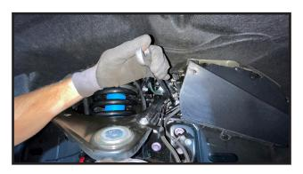
15. Tighten the upper strut mounting hardware. **Torque to** the vehicle back down to the ground. 50 ft lbs. Repeat on passenger side.
