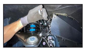
strut 45 degrees to line up to lower strut mount on lower control arm.
