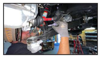
5. Loosen but do not remove. the lower control arm cam bolt hardware on the driver and passenger side.
