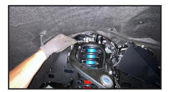
8. Locate the 52220-01 strut spacer's. Install on the top of the struts using OE nuts. The spacer will only fit one way on to the strut. Torque to 45 ft lbs.
