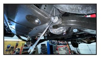
6. Remove the two bolts that attach the the lower ball joint to the bottom of the steering knuckle, Pivot the lower control arm down out of the way.
