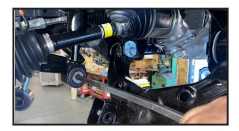
12. Pivot lower control arms back up to the lower struts, Re 16. Re install Sway bar end links to lower control arm. attach to strut using OE hardware. Torque to 140 ft lbs.
