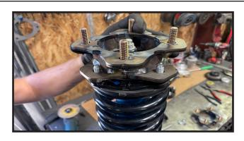
9. Locate the 3/8" flange nuts and re install the strut. Keep the 3/8" flange nuts loose for right now.
