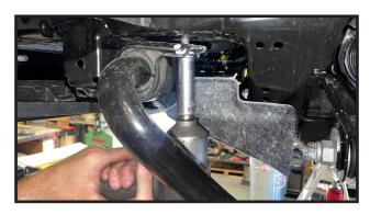
18. Tighten the lower control arm cam bolt hardware on the driver and passenger side. Torque to 150 ft lbs
