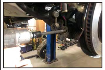
20. Loosen, but do not remove the lower control arm mount-the strut out of the vehicle. ing/adjusting bolts.
