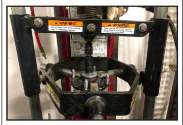
28. Remove the strut from the strut compressor and install (4) S10090 spacer sleeves over the top of the (4) OE upper strut mounting studs.
