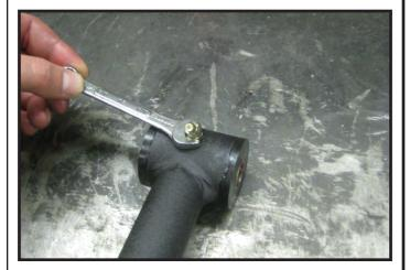
12. Locate (2) S10077 oversized washers, Install the new upper control arm using the oversized washers on the inside bushings. Refer to photo below for location. Torque the OE upper control arm mounting bolt to 125 ft lbs.
