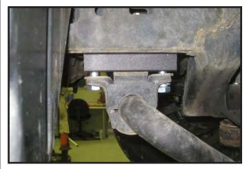
35. Working on the driver side, remove the hardware that attaches the front portion of the differential to the OE mounts. Save the over size washer on the head side of the bolt. Repeat procedure on the passenger side.
