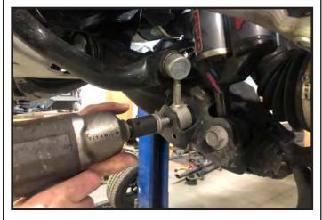
19. Remove the lower strut mounting bolt at the lower control arm.
