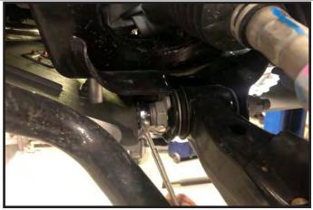
18. Remove the lower bolt where the sway bar endlink atta-21. Remove the bolts that attach the lower control arm to the bottom of the steering knuckle. Make sure to hold onto or support the lower control arm so it does not swing out of control.
