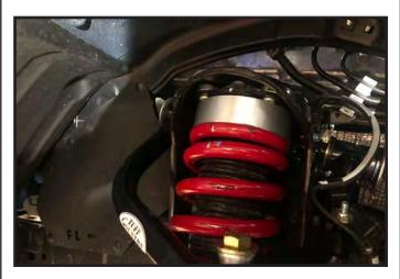
30. Looking at the lower control arm, where the pocket that holds the lower mount of the strut is, you will need to trim the edge of this mount to clear the lower stem of the strut. Refer to below photo for trimming.
