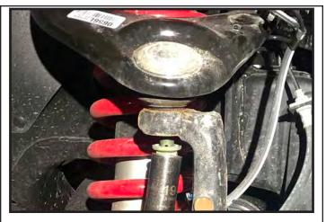
Support the lower control arm using a suitable jack.Carefully strike the top of the steering knuckle with a hammer to to break loose the upper ball joint taper.
