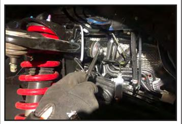
ware, then carefully remove the upper control arm from the (4) TC-002 poly bushings, (2) S10239 crush sleeves, and (2) SERT06 grease fittings. Install the new bushings and sleeves into the new upper control arms. Special note: Make sure to use a fair amount of lithium or moly base grease before installing the new bushings and sleeves into the control arms. This will increase the life of the bushing as well as help prevent squeaking.
