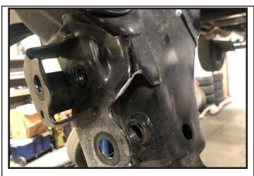
31. Swing the lower control arm back up and pin the lower strut mount using the OE hardware.
