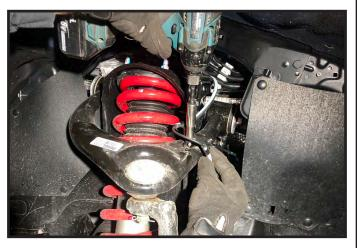
Remove the cotter pin and castle nut from the upper ball joint.
