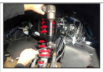
15. Re-attach the ABS wire harness bracket to the new upper control arm using the 1/4" unitorque nut and 1/4" flat washer.
