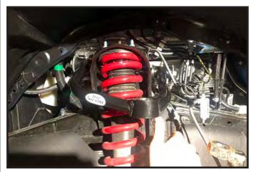
11. Install the new grease fittings into the new upper control 13. If you are installing kit #52080 with ball joint style control
