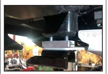
42. Carefully tighten all the skid plate mounting hardware, making sure at the rear most locations to use the OE diamond shaped washers and OE nuts.
