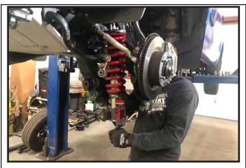
Tuff Country EZ-Ride Suspension recommends a wall mounted strut compressor be used when performing the steps that talk about installing the strut spacer into the strut. If you do not have a wall mounted strut compressor, please have these steps performed by your local Toyota Dealership or certified install shop.
