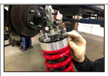
29. Install the strut back into the vehicle using the 4 OE upper mounting nuts. Make sure to only tighten these by hand at this time.
