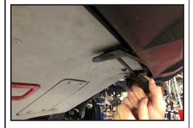
Remove all the front skid plate mounting hardware, including the tow hook bolts. Carefully remove the skid plate and set aside for later work. Refer to the following photo for all attachment points
