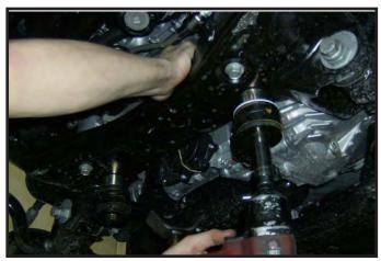
37. Locate the front skid plate and remove all of the OE mounting bolts. There are retainer rings on each bolt that will have to be carefully removed and saved for re-installation.
