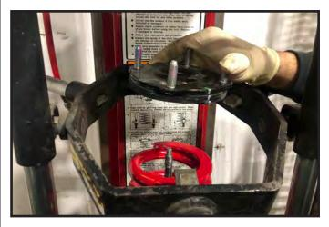
25. Remove and discard the rubber spring isolator from the bearing plate.
