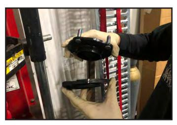
26. Locate the new strut spacer and install the bearing plate on top of the new spacer.
