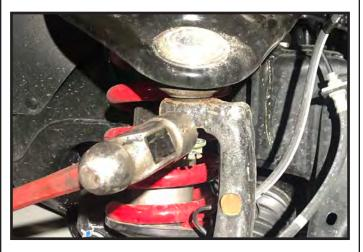
7. Seperate the upper ball joint from the steering knuckle and carefully let the knuckle hang off to the side.
