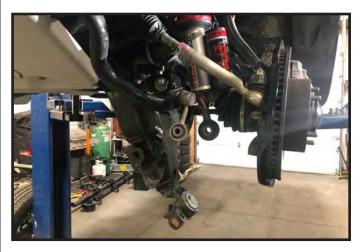
22. Remove the 4th upper strut mounting nut and carefully lift
