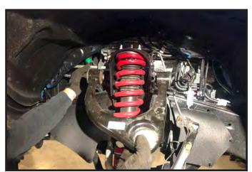
9. Remove the upper control arm mounting bolt and hard-10. Locate the new driver side upper control arm, also locate vehicle.
