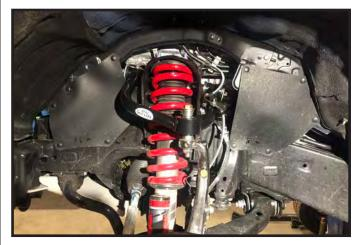
17. Remove the upper strut mounting hardware, but leave 1 of the nuts finger tight to hold the strut in place.
