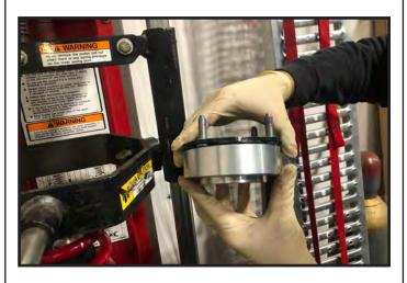
27. Re-install the new spacer and the bearing plate assembly back on top of the coil spring making sure to line up the marks you made previously. Carefully compress the coil until you can re -install the OE bushing, washer, and nut.
