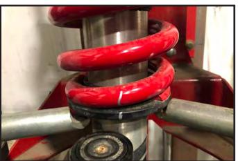
24. Carefully compress the strut until the upper bearing plate can be removed. Remove the nut and hardware from the upper bearing plate and save the hardware for later re-installation. Special note: Notice that on top of the bearing plate there is an arrow indicator marking. This marking is so that the coil over can installed back into the vehicle the same way it was removed, hence the bearing plate needs to be installed the same way it was removed.
