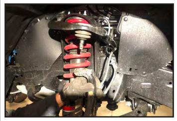
8. Locate and carefully remove the push plugs that are holding the inner fender splash guards to the inner fender, to gain access to the upper control arm bolt.
