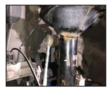
18. Install the front wheels and lower the vehicle to the ground. Torque the lug nuts according to vehicle or wheel manufacturer specifications. Jounce the front of the vehicle up and down a few times to settle the suspension and then torque the upper strut mounting hardware to 30 ft lbs.
