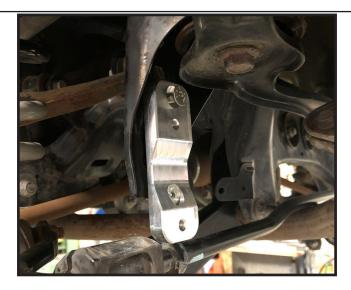
hardware and OE pinch bracket. Make sure to install the pinch bracket with the locking tab facing down. Torque to 25 ft lbs.
