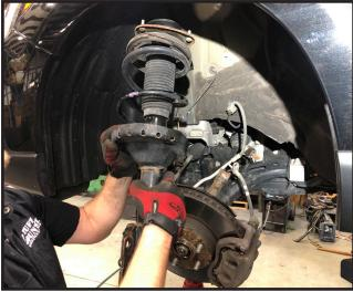
9. With the struts removed from the front of the vehicle, carefully drill the OE upper strut mounting holes out to 3/8".
