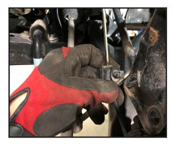
6. Remove the strut to knuckle bolts. Special note: These bolts are specific to upper and lower mounting locations AND direction of install. The upper is a cam bolt, while the lower is a standard bolt. Make sure to note their orientaion for reinstallation later.
