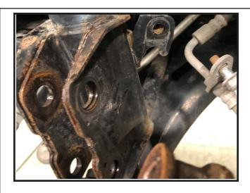
8. Open the hood of the vehicle and carefully support it with the prop rod. Locate the upper strut mounting hardware, and with the help of someone holding the strut, remove the hardware and carefully remove strut assembly from the vehicle.
