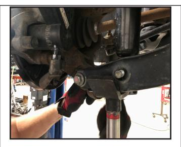
32. Install the front lower control arm to the knuckle using the 34. Install the sway bar to the new brackets using the OE OE hardware. Do not tighten at this time.
