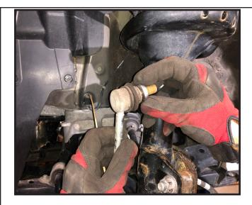
17. Install the sway bar end link on to the new bracket using the OE hardware. Torque the end link and the new bracket to 45 ft lbs.
