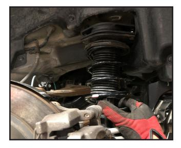
32. Raise the lower control arm into place and install the lower strut hardware. Do not tighten at this time. Use the jack to raise up on the control arm to set pre load on the strut, and install the lower knuckle bolt.
