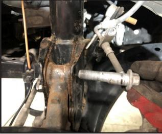
7. While keeping the lower control arm supported, release the knuckle from the strut body and let hang out of the way. Make sure to not over extend the ABS, brake line, and CV axle. Adjust as necessary.
