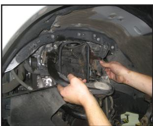
6. Locate the new upper control arms. Locate (8) poly bushings and (4) S10248 sleeves. Install the new bushings and sleeves into the new upper control arms. Special note: Make sure to use a fair amount of lithium or moly base grease before installing the new bushings and sleeves into the control arms. This will increase the life of the bushing as well as help prevent squeaking.
