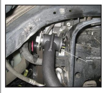
9. Working on the driver side, re-attach the new upper control arm to the steering knuckle using the new castle nut and cotter pin. torque to **90 ft lbs.** Repeat procedure on passenger side.
