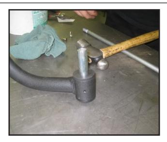
7. Locate the new grease fittings. Install the new grease fittings into the new upper control arms. Special note: Make sure not to over tighten and also make sure that the sert fitting is facing towards the outside of the vehicle. This will make for easier access when using a grease gun.
