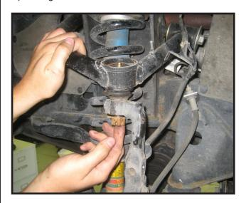
10. Working on the driver side, locate (1) 1/4" nylock nut and (1) 1/4" USS flat washer. Attach the OE ABS brake wire bracket to the new upper control arm. Repeat on passenger side.
