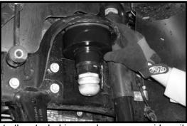
7. Locate the stock driver and passenger side coil springs that were removed in step # 4. Working on the driver side, install the driver side coil spring into the stock location. Repeat procedure on the passenger side. Carefully raise up on both hydraulic floor jacks until the stock coil springs
