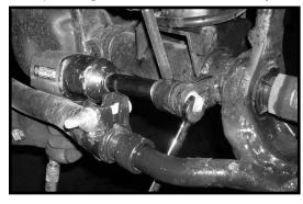
4. Working on the driver side, remove the stock mounting hardware that connects the stock shock into the stock lower mount. Save the stock hardware for later re-installation. Repeat procedure on the passenger side. Special note: There is no need to remove the shock completely from the vehicle. Keep the stock shock mounted to the stock upper mounting location.
