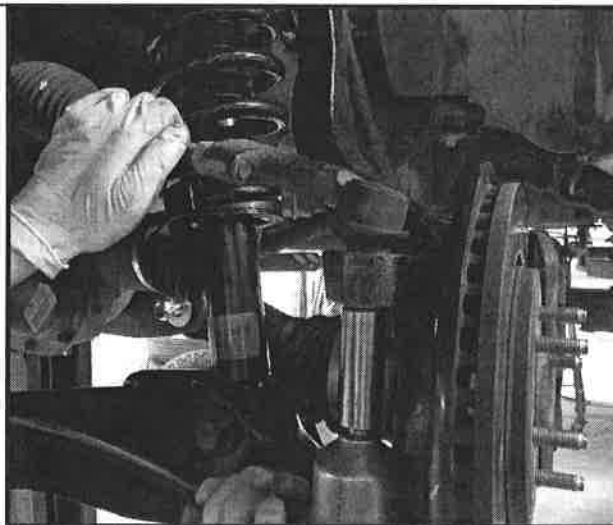
65. Locate the new front drive line spacer and (6) 10mm Allen headed bolts. Install the spacer between the front differential, and the drive line. Special note: Make sure to line the drive line up with the reference mark that was made in step #22.
