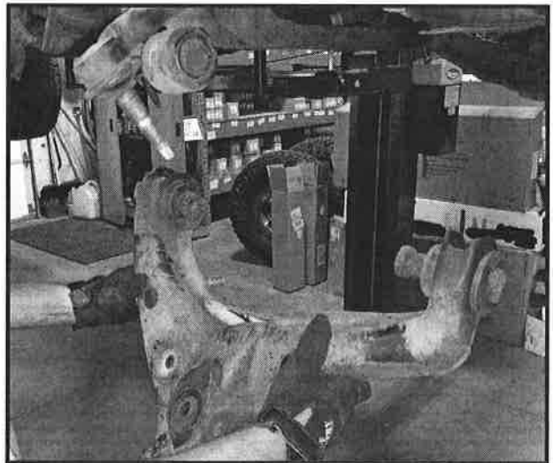
19. Completely remove the sway bar from the vehicle and set out of the way.
