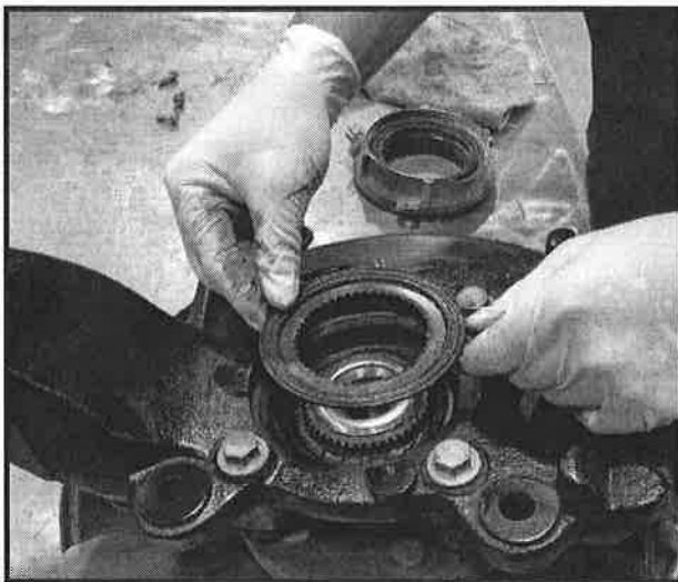
50. Re-install the vacuum actuator in the same order that it was removed and using the OE bolts.
