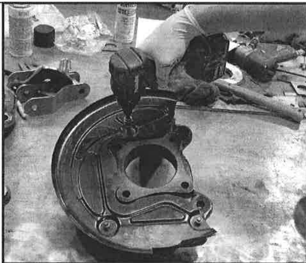
49. Re-install the hub assembly into the new steering knuckle making sure that the hole for the wheel speed sensor is facing upwards.
